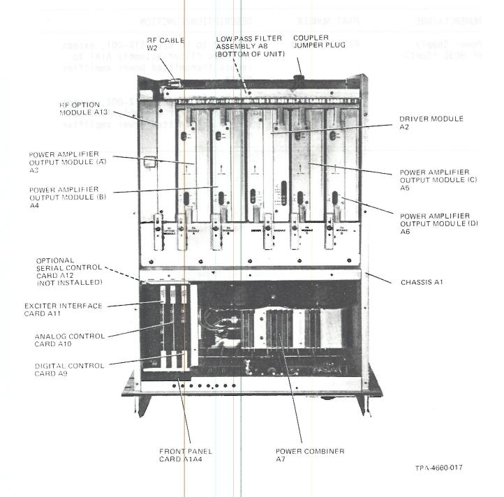
1-kW Power Amplifier HF-8023, Assembly and Subassembly Locations Figure 1-1 (Sheet 1 of 2)
