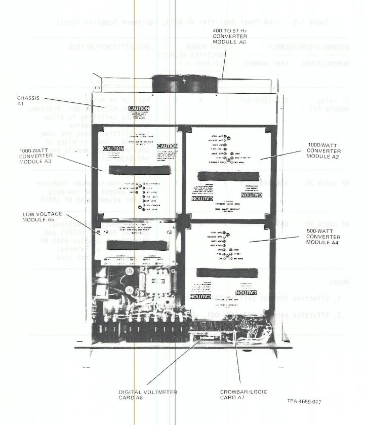
Power Supply HF-8031 and HF-8032, Assembly and Subassembly Locations Figure 1-2 (Sheet 1 of 2)
