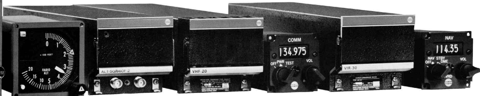
ALT-50 RADIO ALTIMETER —Within 2' or 2% in critical approach phase. Selectable, decision height adjustable over the full range. R-1 3 1 / 2 " x 3 1 / 4 " x 12 1 / 2 ". 7 lbs. $4,890*
